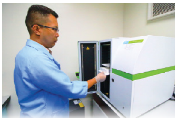
The microplate liquid scintillation counter for receptor binding assay
