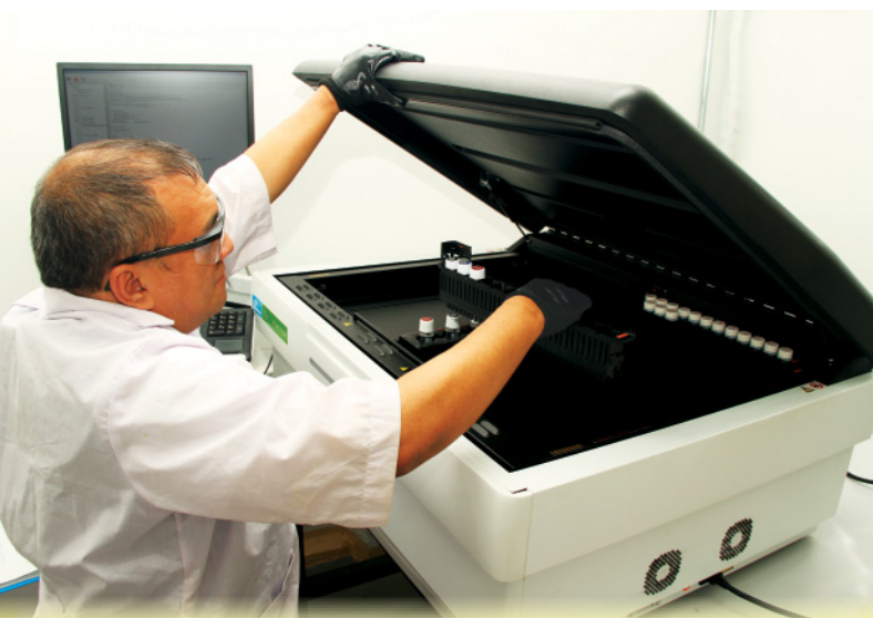
Preparation and analysis of vinegar samples using a liquid scintillation counter
