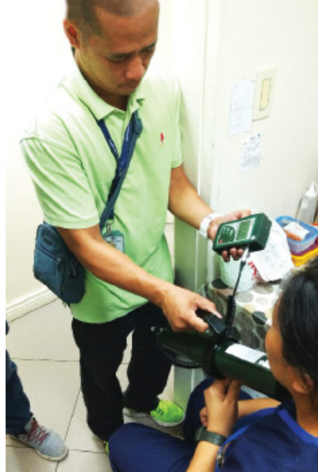
Measurement of radioiodine concentration in thyroid of a nuclear medicine facility staff
