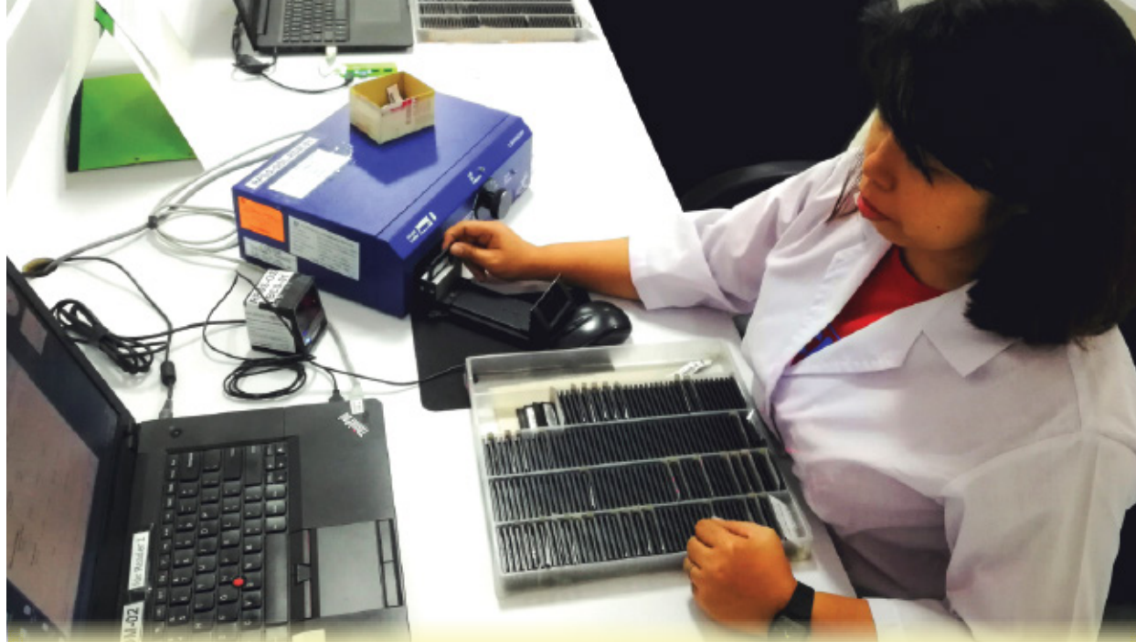
Processing of optically stimulated luminescence (OSL) dosimeters for personnel radiation monitoring
