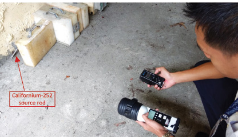
A RIAS personnel measuring the gamma and neutron dose rates coming from a californium-252 source rod.
