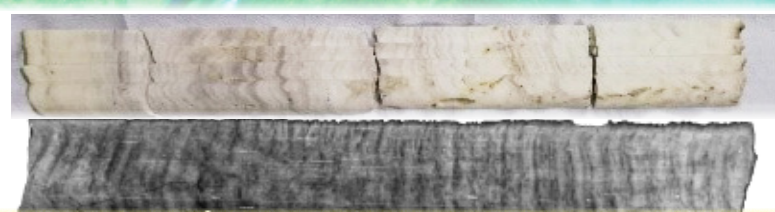
(Top photo) Coral sampling using a hydraulic drill (Middle) Actual image and (Bottom) X-ray image of collected coral cores from Baler, Aurora Province
