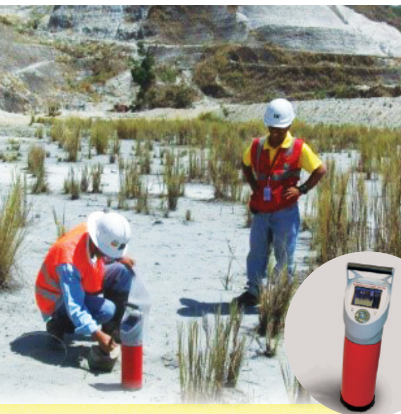
Measurement of uranium concentration using an RS-330 gamma spectrometer (inset) for use in characterization of natural resources
