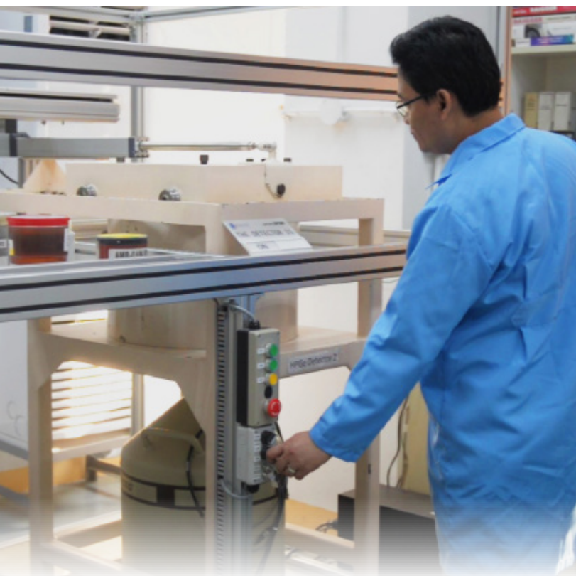
Analysis of food samples by gamma spectrometry at the PNRI Atomic Research Center
