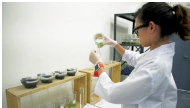
Pretreatment of raw phosphoric acid for uranium extraction
