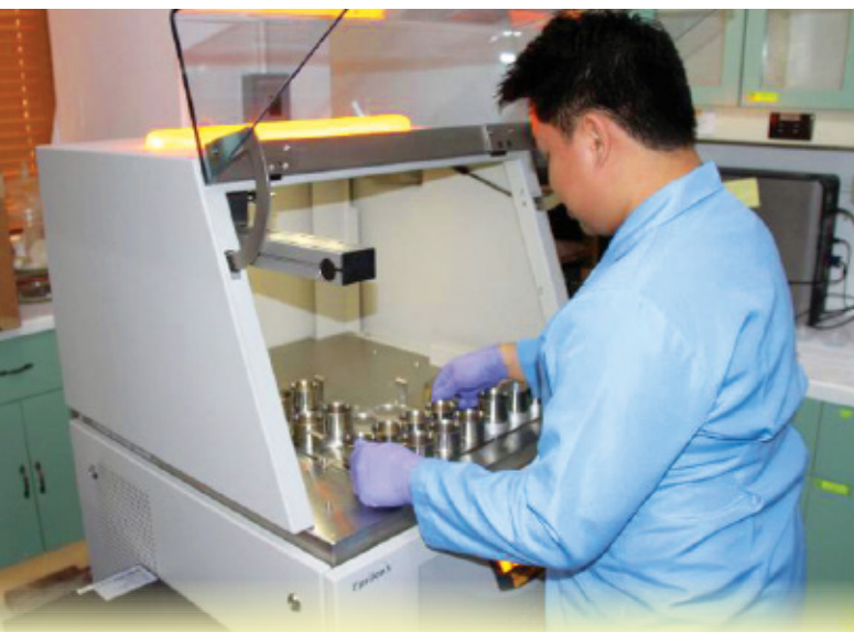
Analysis of air filter samples using the X-ray fluorescence spectrometer
