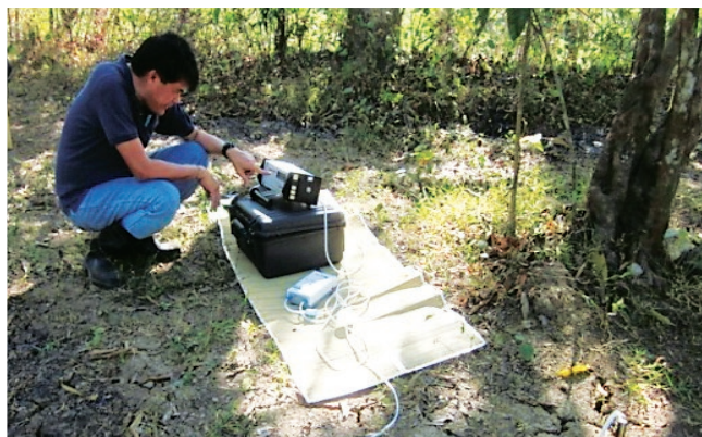
Radon measurement in soil using alphaGUARD radon monitor
