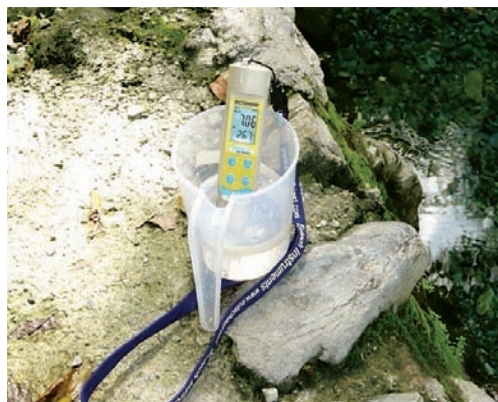
Field geochemical measurement using handheld OAKTON multi-parameter tester
