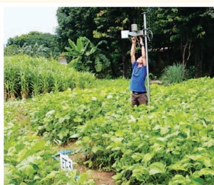
Installation of automatic weather station for agrometeorological data acquisition
