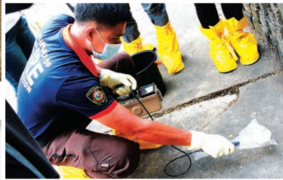
Training course participants perform exercise on surface contamination monitoring and decontamination.
