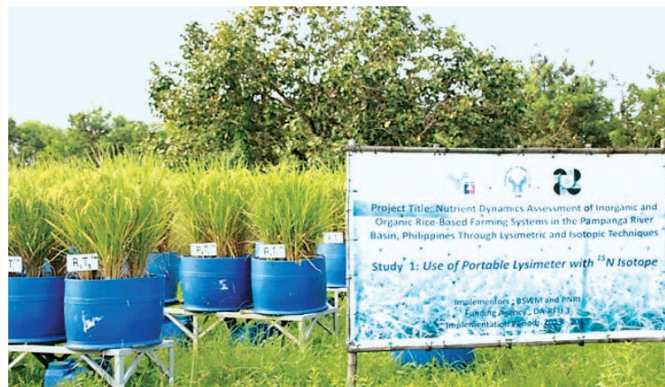
Lysimeters used for studying leaching losses in different fertilization and irrigation management for rice production system
