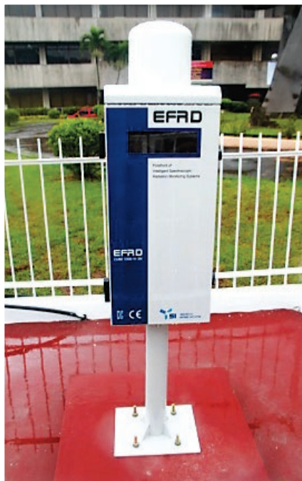
The first real-time radiation monitoring station in PNRI with EFRD 3300 Detector
