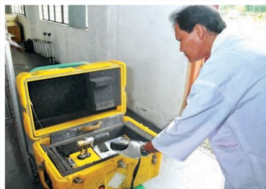
Leak testing of sealed radioactive materials being done by the Radiation Protection Services Section staff
