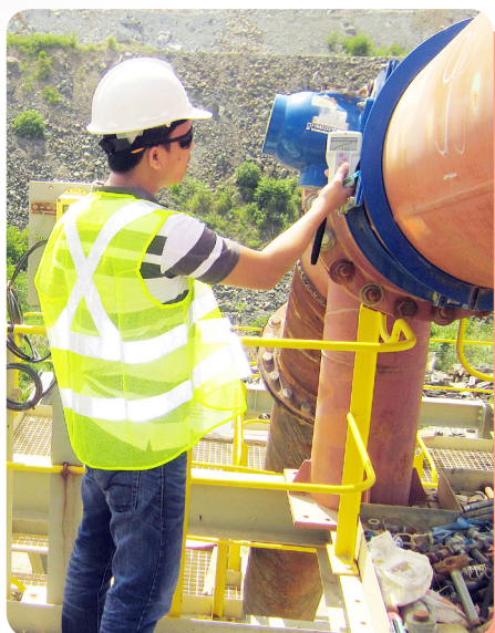
A PNRI inspector verifies radiation levels at a nuclear industrial gauge
