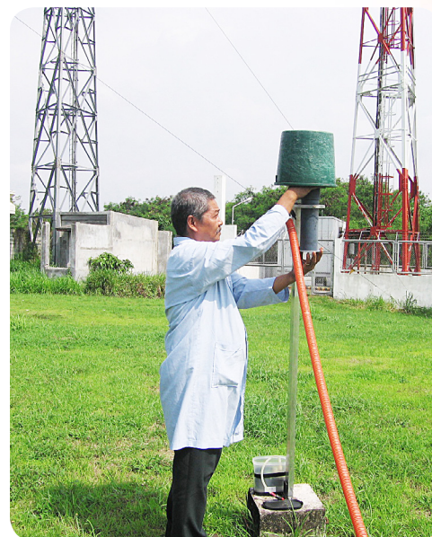
Gent sampler set-up at an air monitoring station
