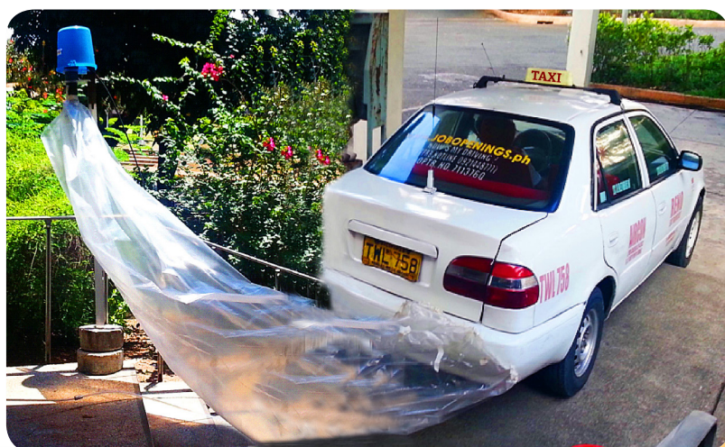
Improvised set-up for the collection of air particulate samples from the tail pipes of vehicles
