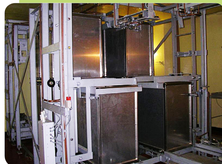
Tote boxes inside the irradiation cell
