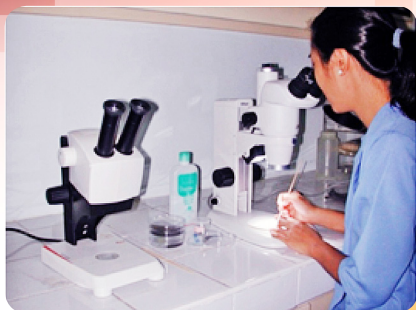
Allanite (center) and monazite (extreme right) mineral grains are separated by hand from bulk samples with the aid of a stereomicroscope (extreme left).
