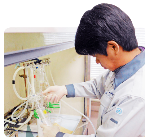
A PNRI research specialist uses the nitrogen gas line to prepare the grafting reaction vessel.
