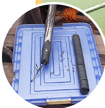
Sediment sampling using suction auger
