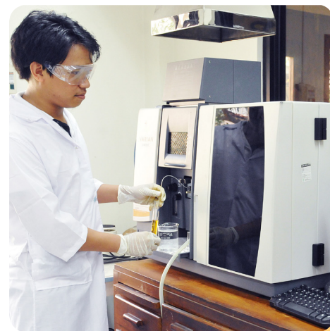
Elemental analysis using the Atomic Absorption Spectrometer (AAS)
