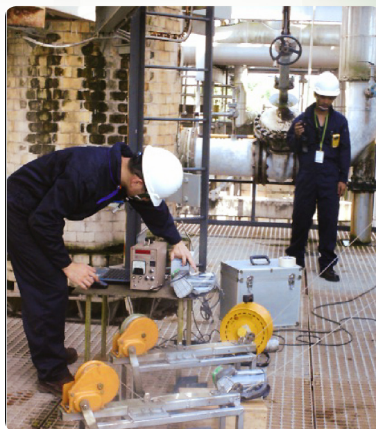
A Science Research Specialist of Isotopes Techniques Section performs gamma-ray scanning at a petrochemical plant.
