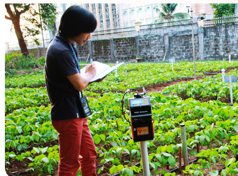
Monitoring and measurement of soil moisture using Soil Moisture Neutron Probe
