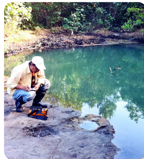
Measurement of potassium, uranium, thorium by gamma ray spectrometry over soil in a hot spring
