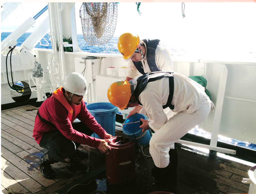
Collection of seawater samples in the West Philippine Sea during the Koyo Maru cruise for the analysis of anthropogenic radionuclides ^{134}\text{Cs} and ^{137}\text{Cs}
