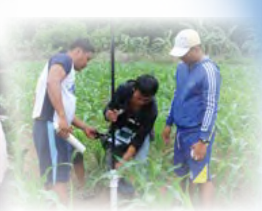
Monitoring of soil water content using automated frequency domain reflectometer
