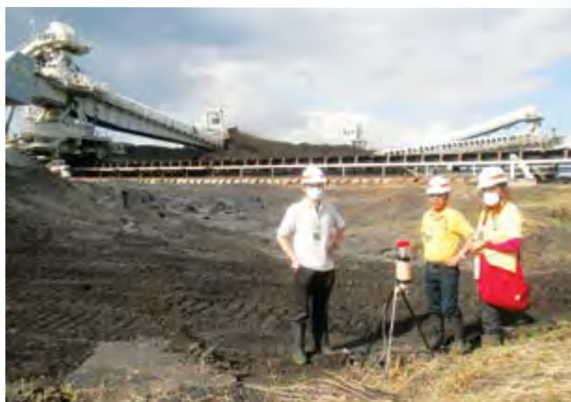
Radiation measurements at coal pit in Pagbilao Coal-fired Power Plant, Pagbilao, Quezon
