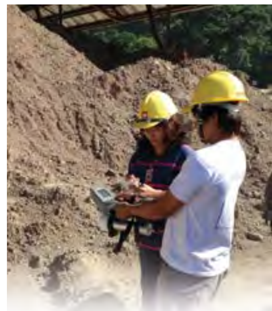
Collection of NORM/TENORM samples and measurement of ambient gamma radiation at Northern Cement Corporation, Sison, Pangasinan
