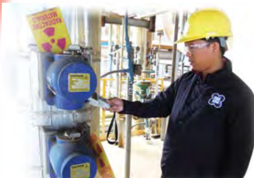
PNRI inspector verifies the radiation level of a nuclear industrial gauge
