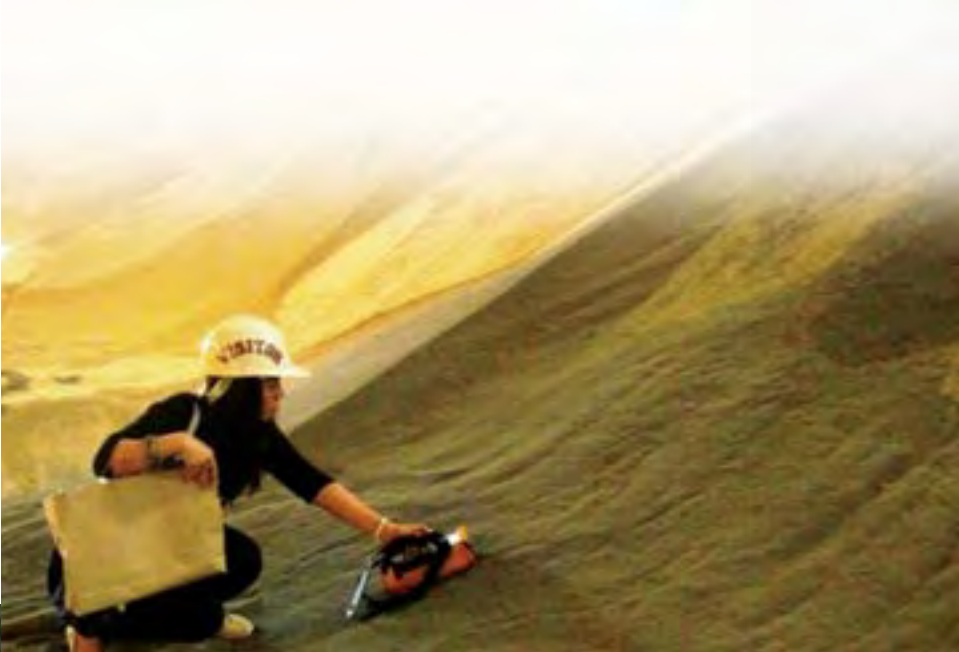
In-situ gamma measurement of phosphate rock storage area in Philphos, Isabel, Leyte with the use of a portable gamma spectrometer
