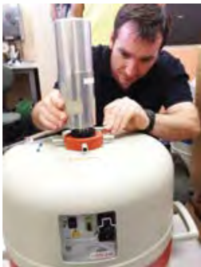
Mr. Guillaume Beziat, CTBTO Engineering Development staff installs the Canberra Cryo-cycle Hybrid Cryostat for the HPGe detector at RN52 Station in Tanay, Rizal.
