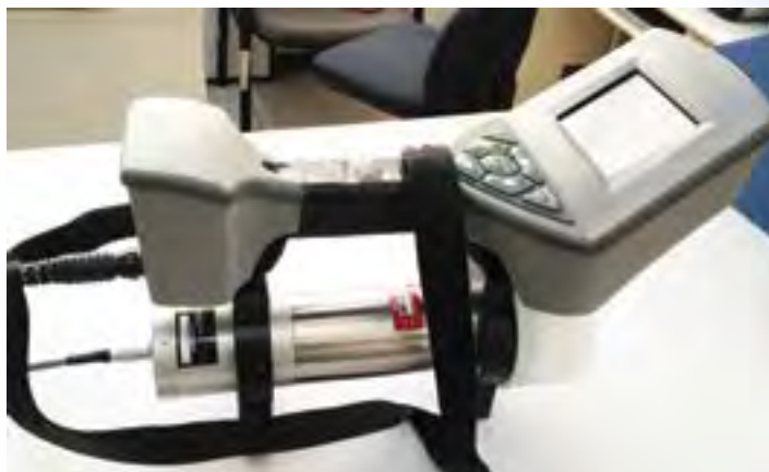
SAM 940 portable isotope identifier used for ambient gamma radiation measurements
