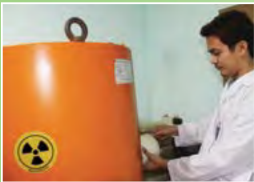
Samples are placed inside the Neutron Calibrator for neutron activation analysis
