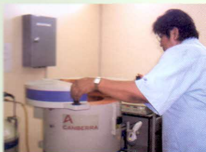
A Germanium detector inside the CTBTO PHP52 station in Tanay, Rizal is used for counting of radioactivity levels of air filter samples.
