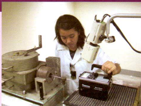
A staff from the Radiation Protection Services sets up a survey meter for response tests and calibration at the PNRI Secondary Standards Dosimetry Laboratory.
