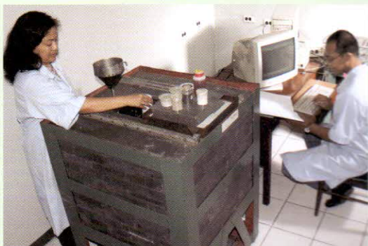
Counting of radioactivity levels of phosphate rock samples from Philphos using HPGe detector
