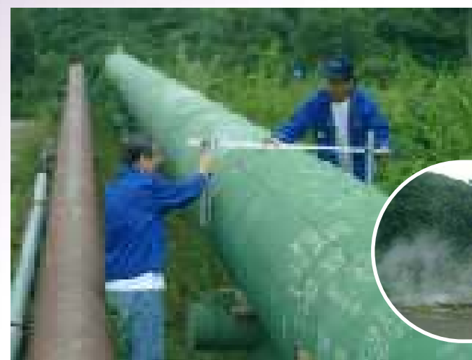
PNRI uses a nuclear technique to measure deposition of solids in walls of pipelines at the geothermal facility in Tongonan, Leyte.
