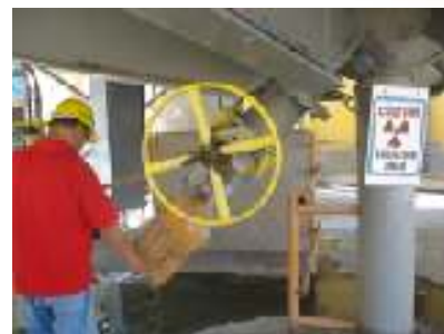
Radiation monitoring of a nuclear density gauge installed at thickener underflow line of Lepanto Consolidated Mining Corporation, a PNRI licensee
