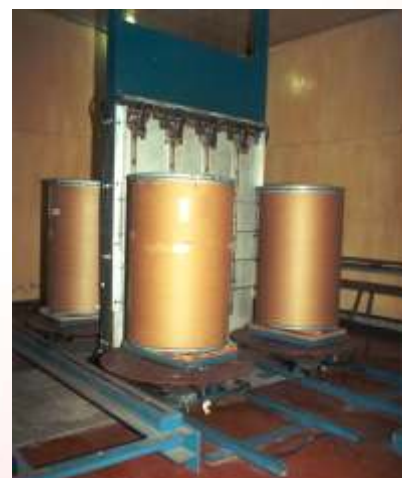
Spices contained in drums are being irradiated inside the Cobalt-60 Multipurpose Irradiation Facility for microbial decontamination.
