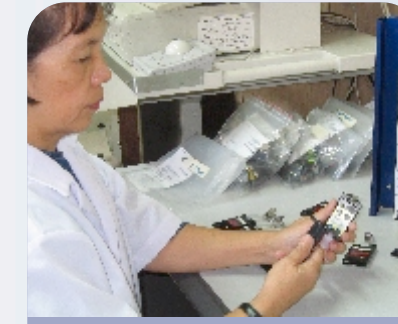
Processing of thermo-luminescent dosimeters for radiation dose evaluation
