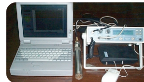
A counting electronic device used in gamma column scanning and pipeline deposit measurement
