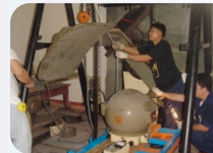
Decommissioning of a disused teletherapy machine in Iloilo
