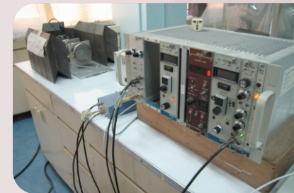
The Moessbauer spectrometer with a new transducer and drive system
