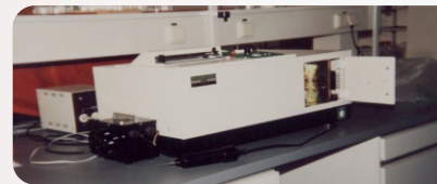
The Jasco N-15 emission spectrometer used for N-15 determination
