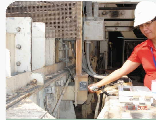
LRE head verifies radiation levels during removal of depleted sealed sources from weighing devices in a coal-fired thermal power plant.
