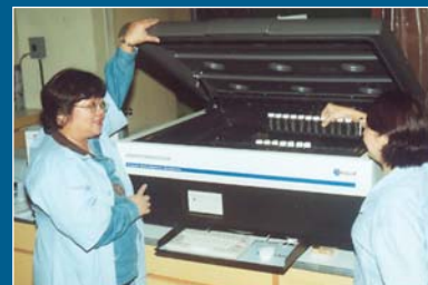
PNRI researchers use the liquid scintillation counter for analysis of water and vinegar samples.
