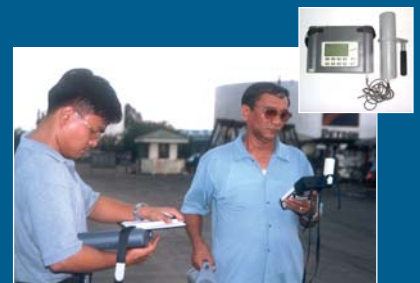
PNRI researchers measure ambient radiant dose rate at Poro Point Communication Facility in La Union using a portable spectrometer (inset)
