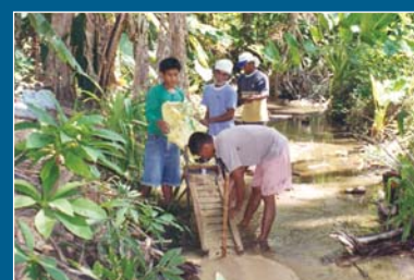
Recovery of heavy minerals in San Vicente, Palawan using a sluice box
