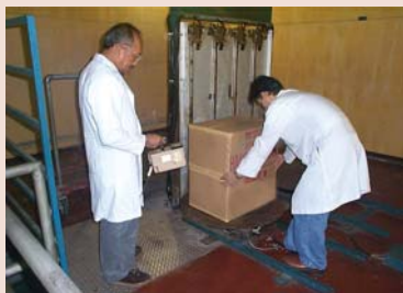
Spices contained in cartons are exposed to gamma radiation inside the cobalt-60 multipurpose irradiation facility for microbial decontamination.
