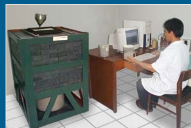
Cesium-137 activity measurement in soil samples obtained in the field by gamma spectrometry
