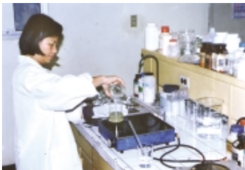
Preparation of hydrogel from carrageenan and polyvinyl pyrrolidone (PVP)
