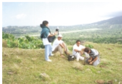
A PNRI researcher (standing) takes the location of the sampling station using the global positioning system while gamma ray measurements are going on.
