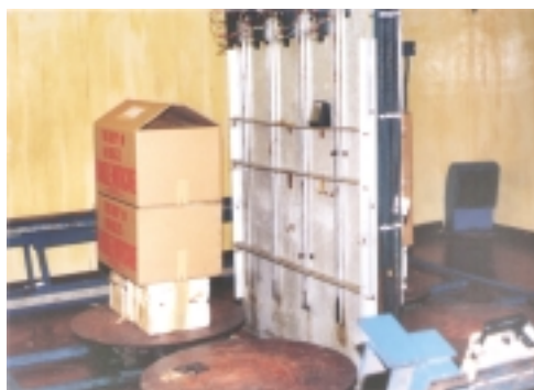
Fruit fly pupae contained in boxes are exposed to gamma radiation inside the cobalt-60 multipurpose irradiation facility to make them sterile.
