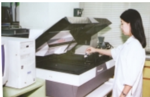
Carbon-14 measurement of vinegar samples using liquid scintillation counting
