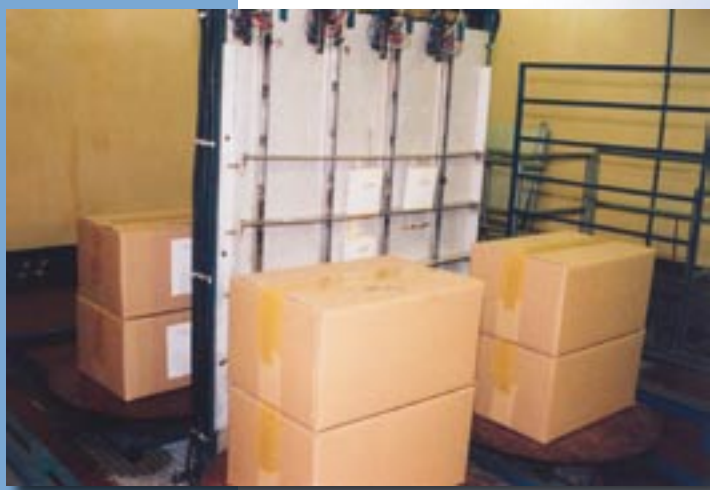
Spices contained in carton boxes are exposed to gamma radiation inside the cobalt-60 multipurpose irradiation facility for microbial decontamination.
