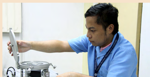
Researchers preparing honey samples for analysis using an Isotope Ratio Mass Spectrometer (IRMS)
