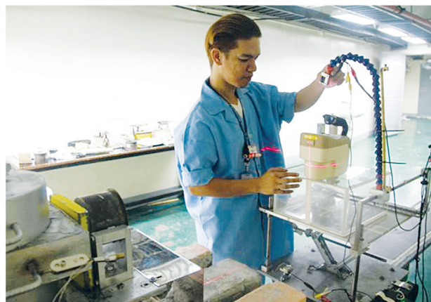
Calibration of a survey meter in the Secondary Standards Dosimetry Laboratory
