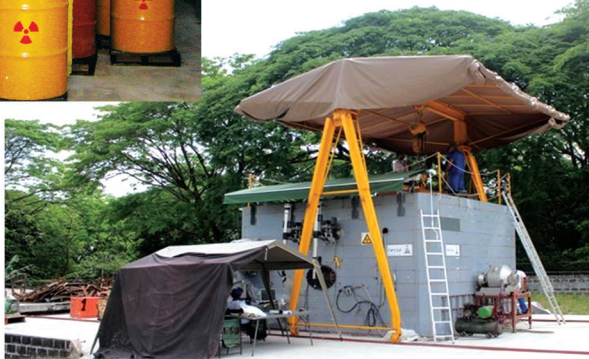
An assembled mobile hot cell for conditioning Spent High Activity Radioactive Sources
