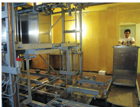
The irradiation room and storage transport system of the Co-60 Multipurpose Irradiation Facility
