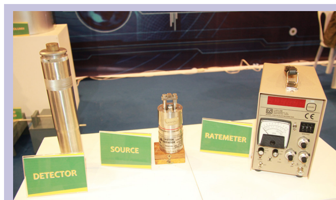
Some equipment used for gamma column scanning
