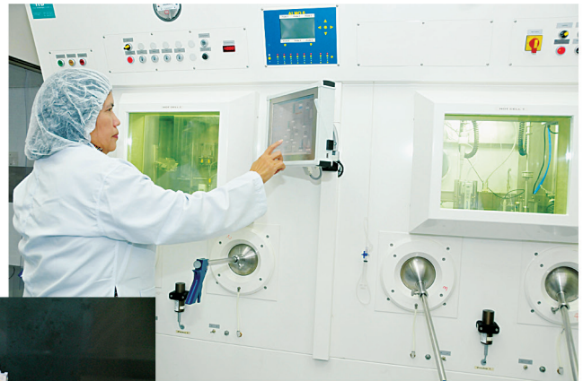
The Tc-99m hot cell facility inside the Radioisotope Laboratory building.
