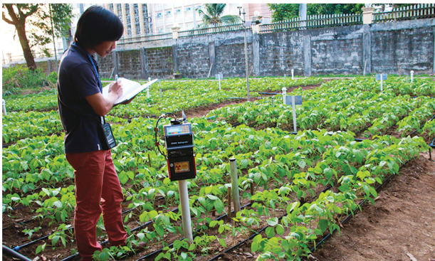
Monitoring and measurement of soil moisture using Soil Moisture Neutron Probe
