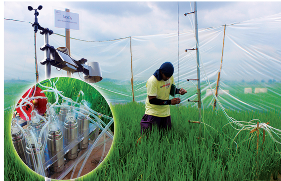
Fabrication and testing of air moisture sampling device for partitioning soil water evaporation and crop transpiration
