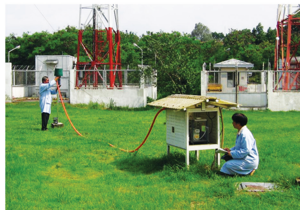
Gent Sampler set-up at an air monitoring station
