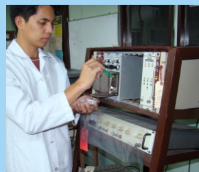
Loading of samples in alpha particle counter for lead-210 dating analysis
