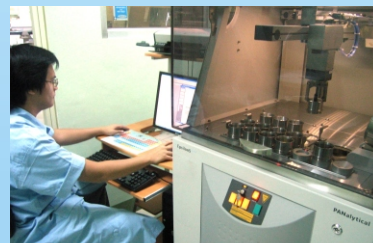
Multi-element analysis of air particulate matter using energy dispersive XRF spectrometry
