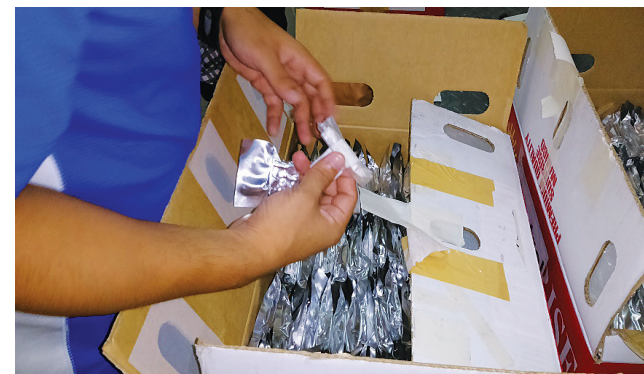
Placing of dosimeters in each box prior to irradiation at the Cobalt-60 Irradiation Facility
